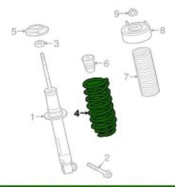
Part or sub-assembly is #4 in diagram Diagram may not be specific to your vehicle
