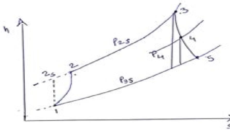
Here, the enthalpy is  $h$ , the entropy is  $s$ , the stagnation pressure at compressor inlet and outlet are  $\rho_{2s}$  and  $\rho_{3s}$  respectively, the stagnation pressure at state 4 is  $\rho_{4s}$ , and 02s is stage state.
